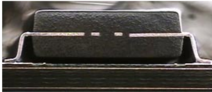
Figure 1 shows cross-sectional over view of U6 with left and right gull wing leads, board 3 ~12x
