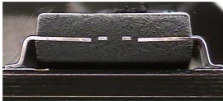
Figure 1 shows cross-sectional over view of U6 with left and right leads, board 1 ~12x
