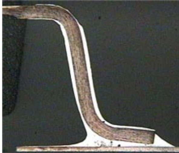
Figure 3 shows a solder joint formation of the right lead. 50x
