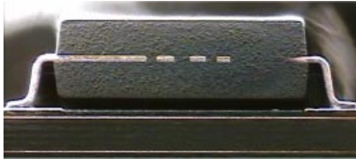
Figure 1 shows cross-sectional over view of U6 with left and right leads, board 2. ~12x
