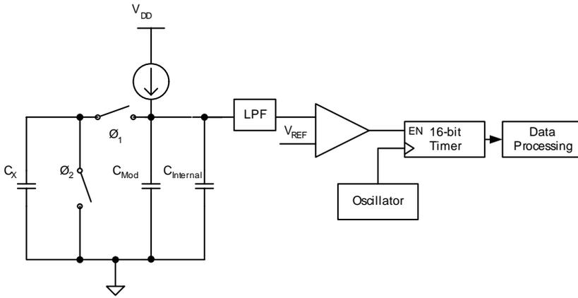
The circuitry brings the sensor capacitor to a voltage relative to the capacitance of the sensor. The PSoC's internal main oscillator (IMO) clocks the switched capacitor.
