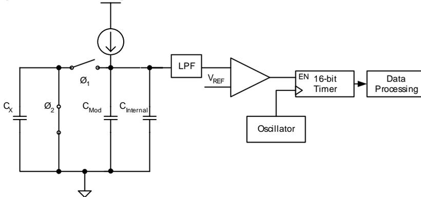
$C_X$  is an effective resistance to ground through phases 1 and 2. An equivalent block diagram is shown in Figure 6. The equivalent resistance is given by:
