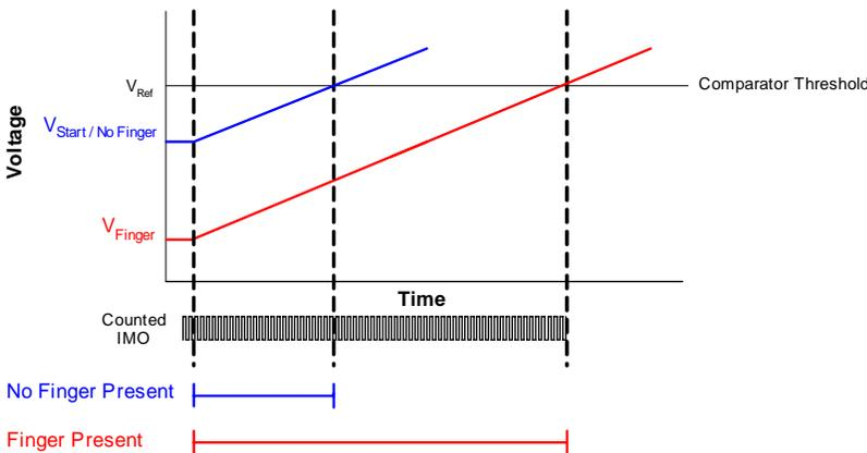
Figure 8. CSA Waveform Seen at Cmod with Finger Present
