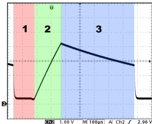
In Figure 8, the starting voltage in region 1 has dropped. This is due to the decrease in equivalent resistance, which itself is a result of the finger capacitance ( $C_F$ ) added in parallel with the sensor capacitance ( $C_X$ ). The charge time in region 2 is longer, resulting in more counts on the counter compared to no finger present on the sensor. An increase in charge time can be seen by comparing Figure 3 and Figure 8.
