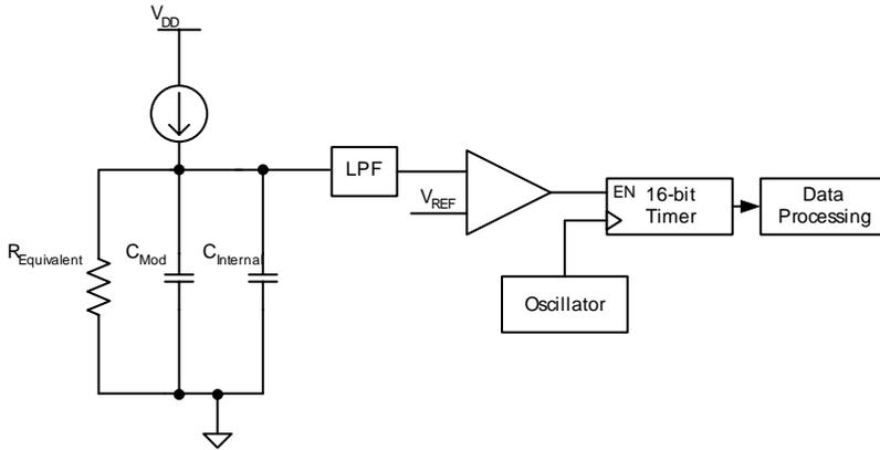
$V_{Start}$  is set to a value below  $V_{REF}$  with the switched capacitor circuit running. This is accomplished by tuning the iDAC through successive approximation, which uses a binary search to determine the appropriate iDAC setting. Once the bus has been charged to  $V_{Start}$ , the iDAC current setting that was used is stored, and the process is repeated for each sensor in the project.
