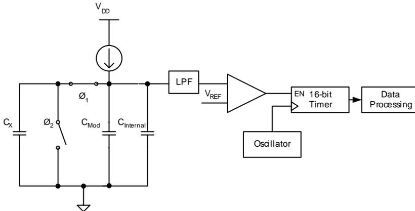
Phase 2 ( $\phi_2$ ) disconnects  $C_X$  from the analog global bus and discharges  $C_X$  by connecting it to ground, leaving only  $C_{Mod}$  and  $C_{Internal}$  connected. This is shown in Figure 5.
