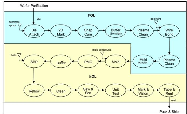
Fig 9 "TRAILER" Process Flow
