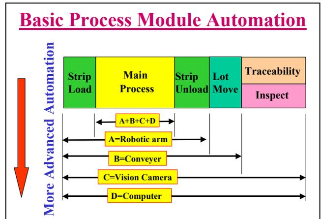
Fig 1 : Equipment Basic Functionality
