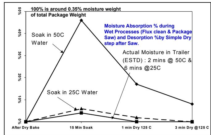
Fig 11: Moisture Absorption after PMC
