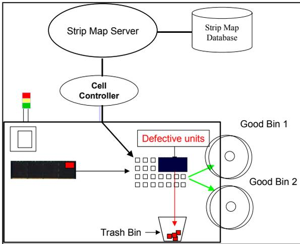
Fig 7: Reject sorting after Singulation
