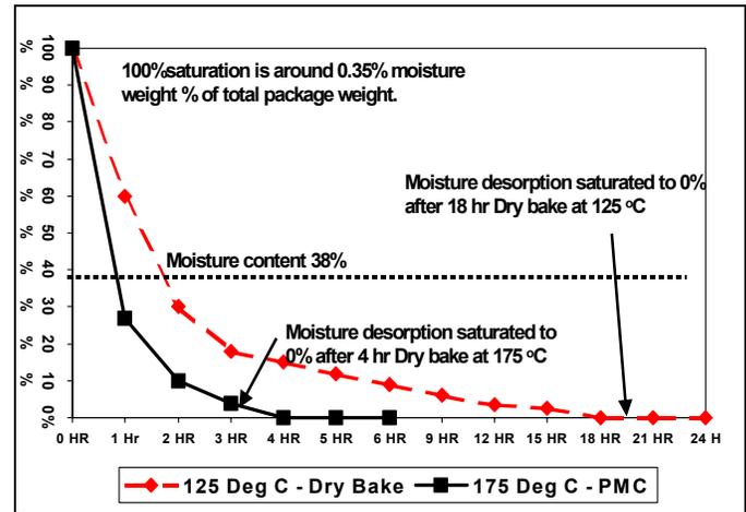
Fig 10: Moisture Desorption Comparison during Dry-Bake and PMC.
