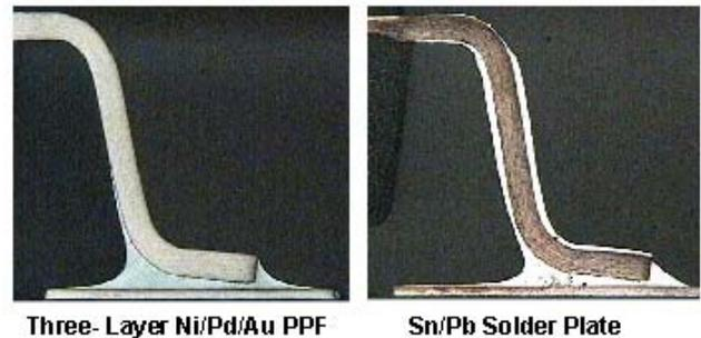
Figure 9: Solder Joint Formation
