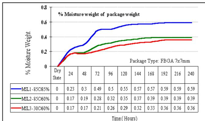
Figure 11: Moisture Absorption Curve by MSL
