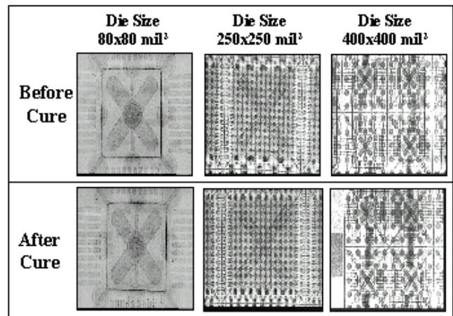
Figure 3: FBGA- Die Size vs Voids After Cure
