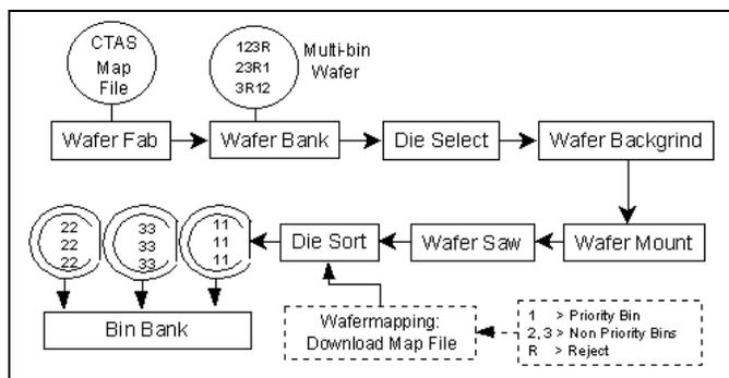
Figure 10: Die Purification Flow
