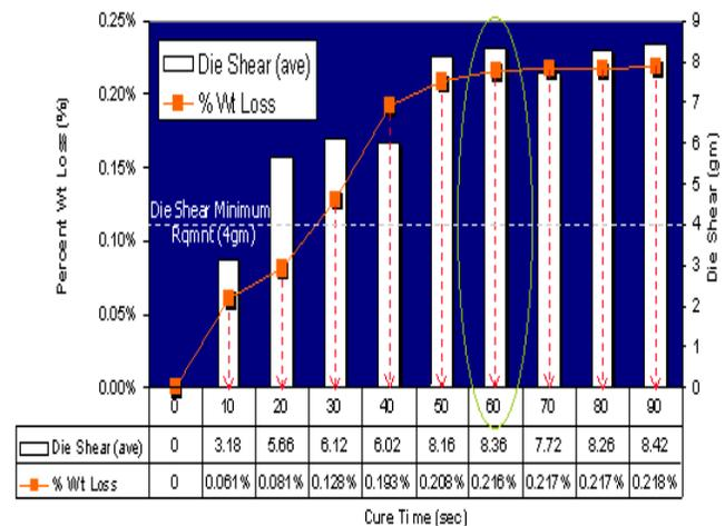
Figure 4: Weight Loss/Die Shear vs Cure Time Study
