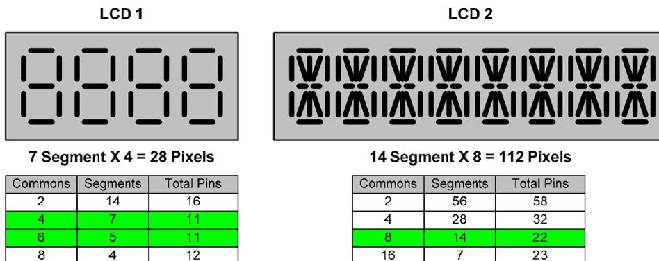
**Figure 3 - Custom LCD Comparison**
