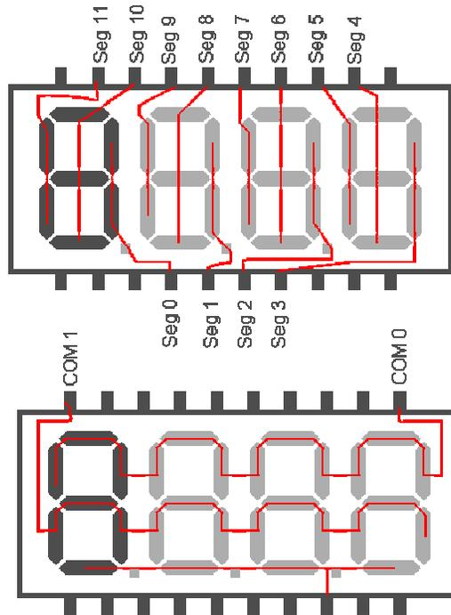
**Figure 2 - Segment and Common Pin Connections in an LCD**
