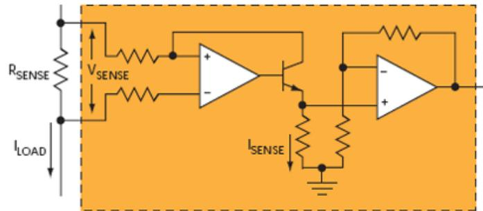
3. A two-stage CSA amplifies the differential high-side voltage while providing ground-referenced feedback to the hysteretic controller.
