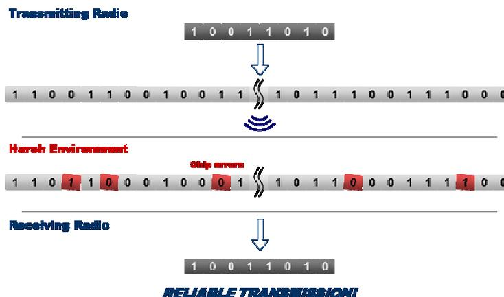
Figure 1 - Example of DSSS principles in use to encode bits of data
