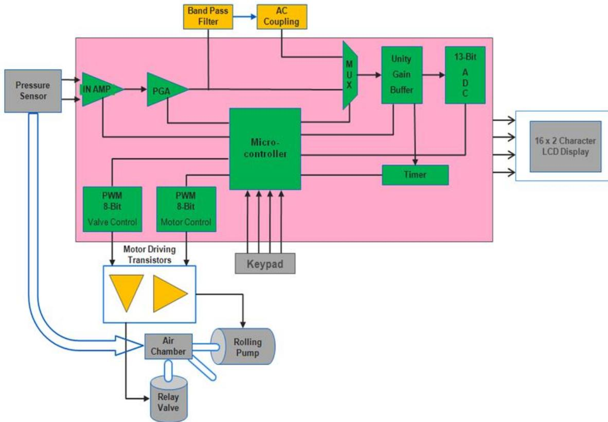
**Figure 1. Blood Pressure Monitor using PSoC**
