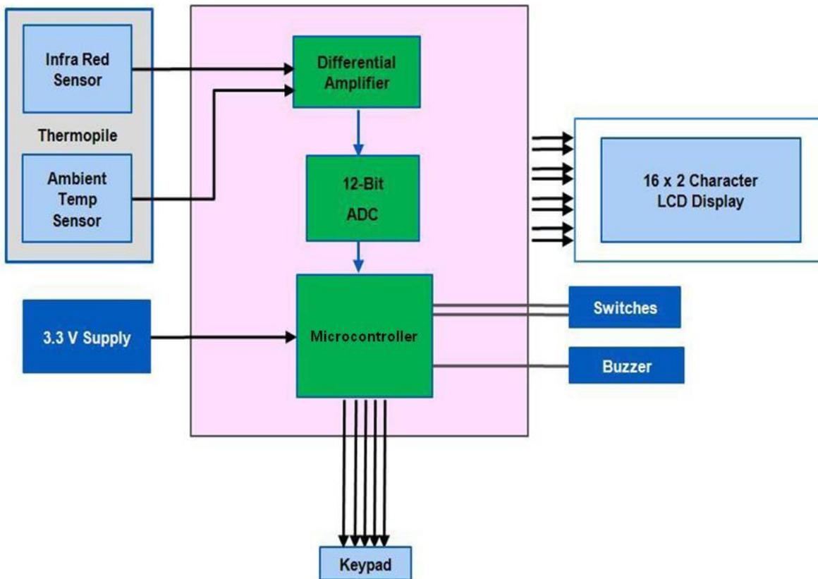
**Figure 3. IR Thermometer using PSoC**
