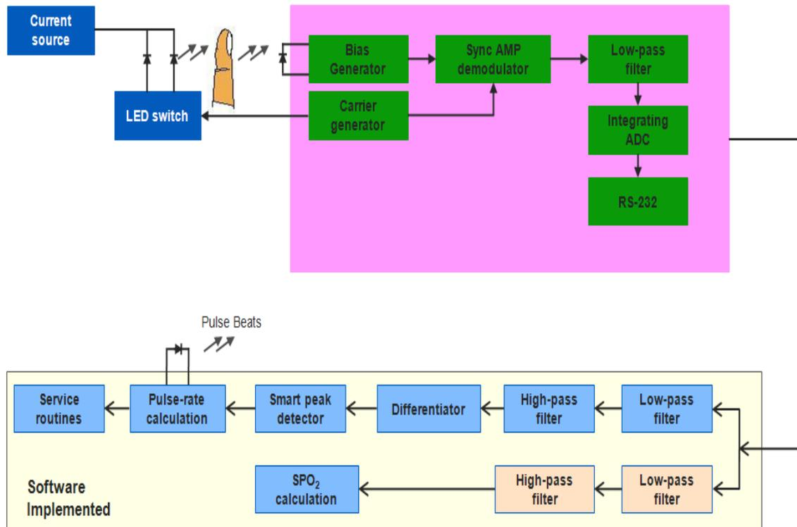
**Figure 2. Pulse Oximeter using PSOC**
