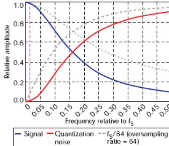
2. In second-order DSMs, the relative amplitude of the signal and quantization noise can be plotted as a function of frequency.
