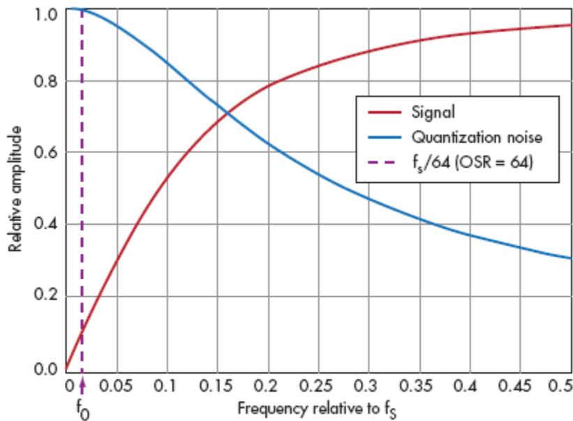
2. As a DSM's noise frequency relative to  $f_s$  increases, the quantization noise's relative amplitude increases, while the signal's relative amplitude decreases.
