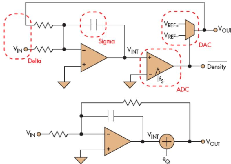
Suppose the references are  $\pm 1$  V. A 0.1-V integrator output results in a 1-V quantized output. This can be seen as 0.1 V with a 0.9 quantization error. A quantized  $-0.3$  is  $-1$  V or the addition of a  $-0.7$ -V quantization error. Bearing this in mind, a DSM can be considered an integrator with a quantization noise source added to its output. Figure 1 shows this model of quantization noise.
