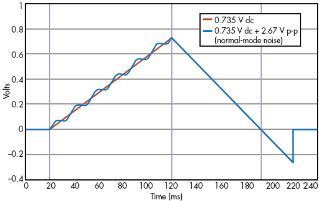
2. A dual-slope converter with a specific integration time can be used to remove mains noise.
