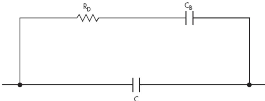
3. Dielectric absorption has a significant effect on the capacitor.
