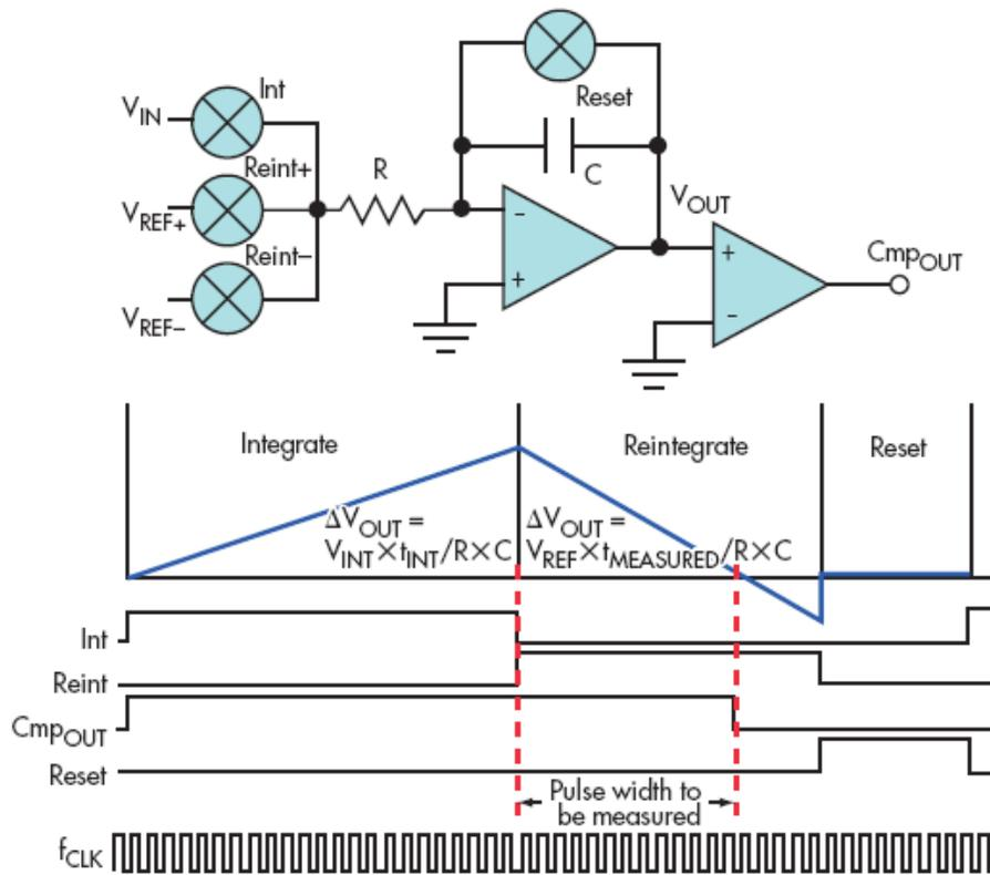
1. With a dual-slope converter, the input and reference voltages pass through the same integrator.
