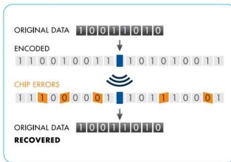
**Figure 1 - Direct Sequence Spread Spectrum**
