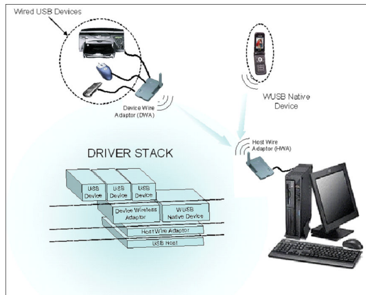
Figure 5. Hardware and Software Stack for Wireless USB System with Wired USB Devices Connected.
