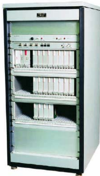
Figure 3: A typical RTU
