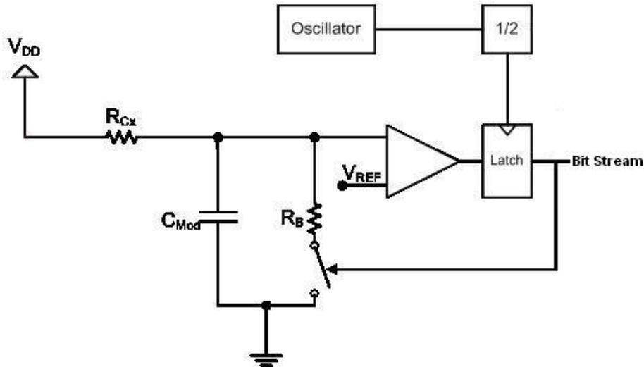
The switch capacitor block, when running, functions as a resistor as shown in Figure 6. The equivalent resistance is calculated by:
