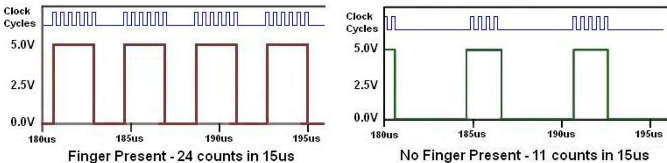
The raw number of clock cycles (referred to as 'counts') from the counter are updated to a register used by the CSD algorithm for determining a finger's presence, as well as setting the baseline and adapting to environmental conditions. The CSD algorithm looks at several measurement windows for each sensor depending on user settings.
