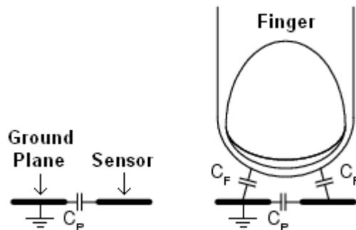
Each sensor is a capacitor with one contact grounded, and the other contact connected to the PSoC's analog global bus. The result is an active variable capacitor,  $C_X$  ( $C_X = C_P + C_F$ ). The presence of a conductive object (such as a finger) increases the capacitance of the sensor with reference to ground. Determining sensor activation is then a matter of measuring the change in capacitance.
