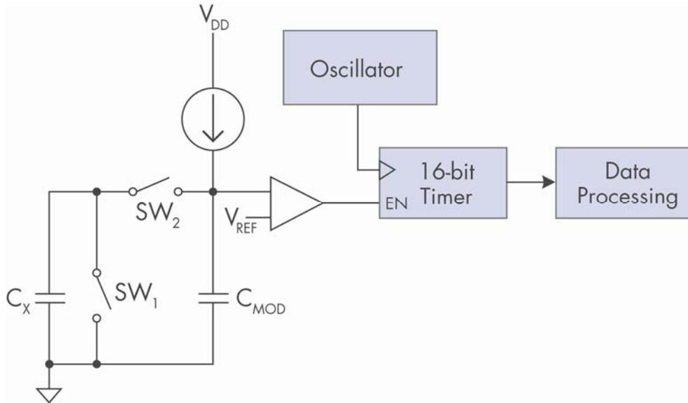
The capacitance to voltage converter is implemented with switched capacitor technology. The circuitry brings the sensor capacitor to a voltage relative to the capacitance of the sensor. The switched capacitor is clocked by the PSoC's internal main oscillator.
