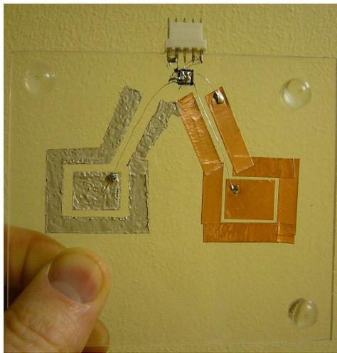
**Figure 3. Close-up view of the copper tape construction. The outer ring is ground, and the inner square is the sensor pad. The wire is a jumper back to the PSoC.**
