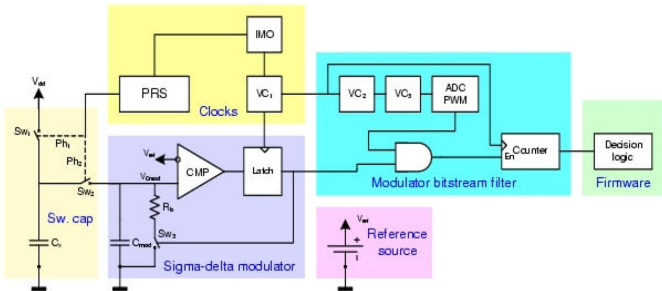
An equivalent circuit of CSD is shown in Figure 5. The switches on the front end of the circuit have turned the sensor capacitance into an equivalent resistance that is modulated by the presence of a finger. The change in the resistance results in variation in the bit stream at the output of the sigma-delta modulator.
