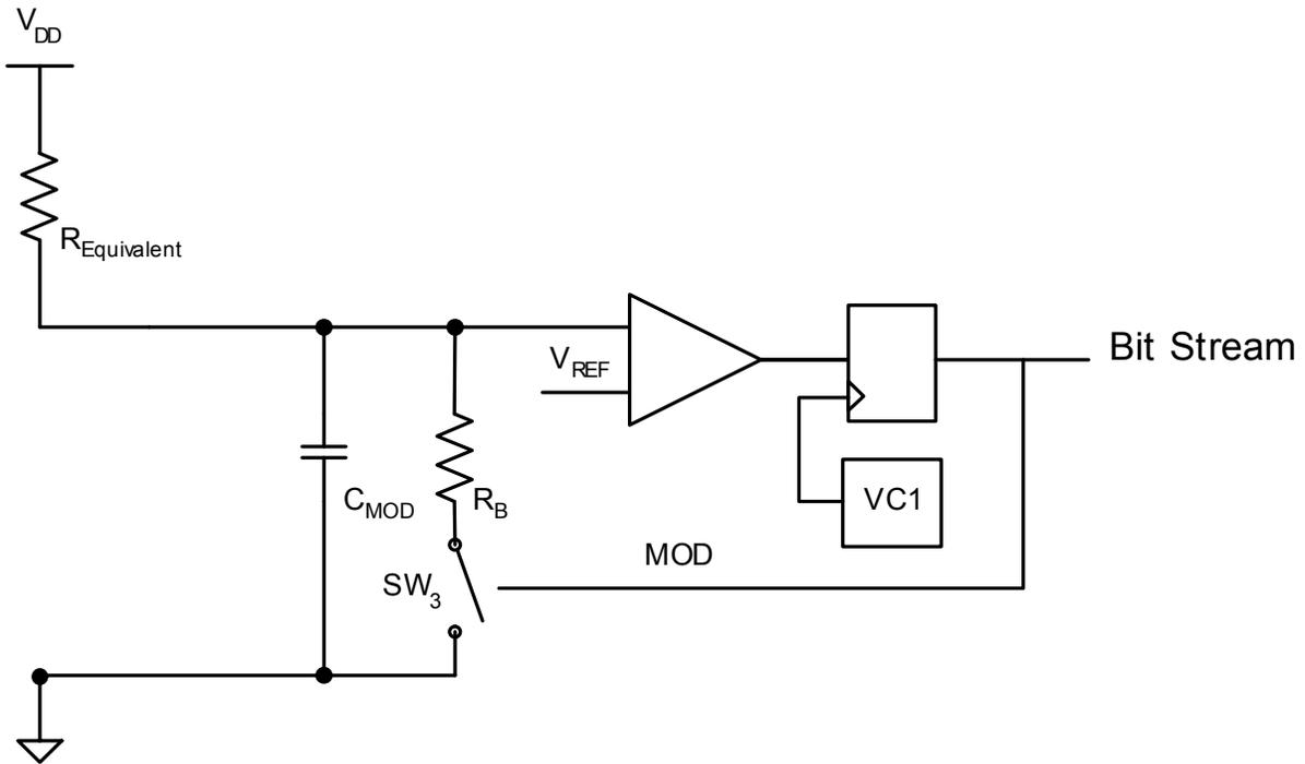
The CSD User Module is a standard functional block included in the PSoC Designer library. It contains API routines that perform all the low level and high level functions required to make a practical capacitive sensing system. The PSoC is selected by dragging-and-dropping the CSD User Module from the library. The system level operation of the sensors is defined in C.
