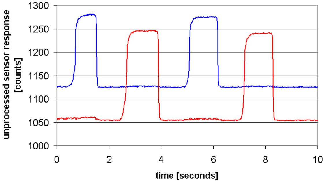
Figure 8. Digital states for the two sensors with a 3mm acrylic overlay. Upper trace is for silver ink. Lower trace is for copper tape.
