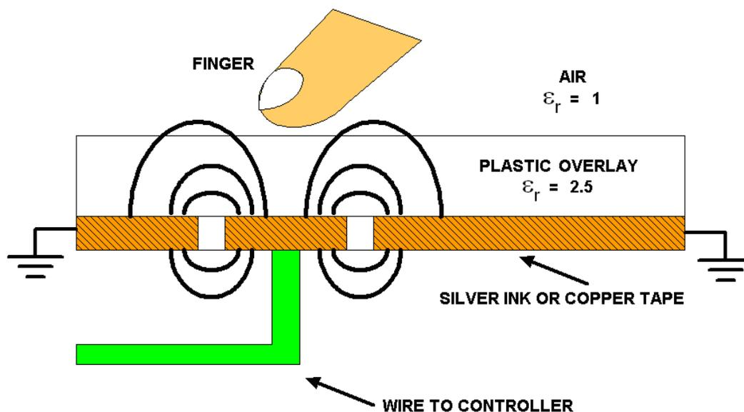
Silver ink pens and copper tape provide a prototyping solution for capacitive sensing that is both inexpensive and quick to implement. A cross-sectional view of the concept is shown in Figure 1. Conductive patterns are applied by hand, directly to the nonconductive overlay material. Jumper wires connecting the microcontroller to sensor pads replace PCB traces of the more traditional approach to prototyping.
