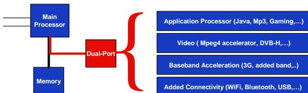
**Figure 1. Upgrading an Architecture by Connecting a Dual-Port on an Existing Memory Bus**
