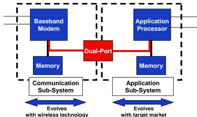
**Figure 2. Defining Different Subsystems with Independent Evolution using a Dual-Port**
