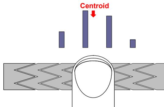
With sliders it is important to choose a sensor shape that easily allows the finger to affect multiple sensors.
