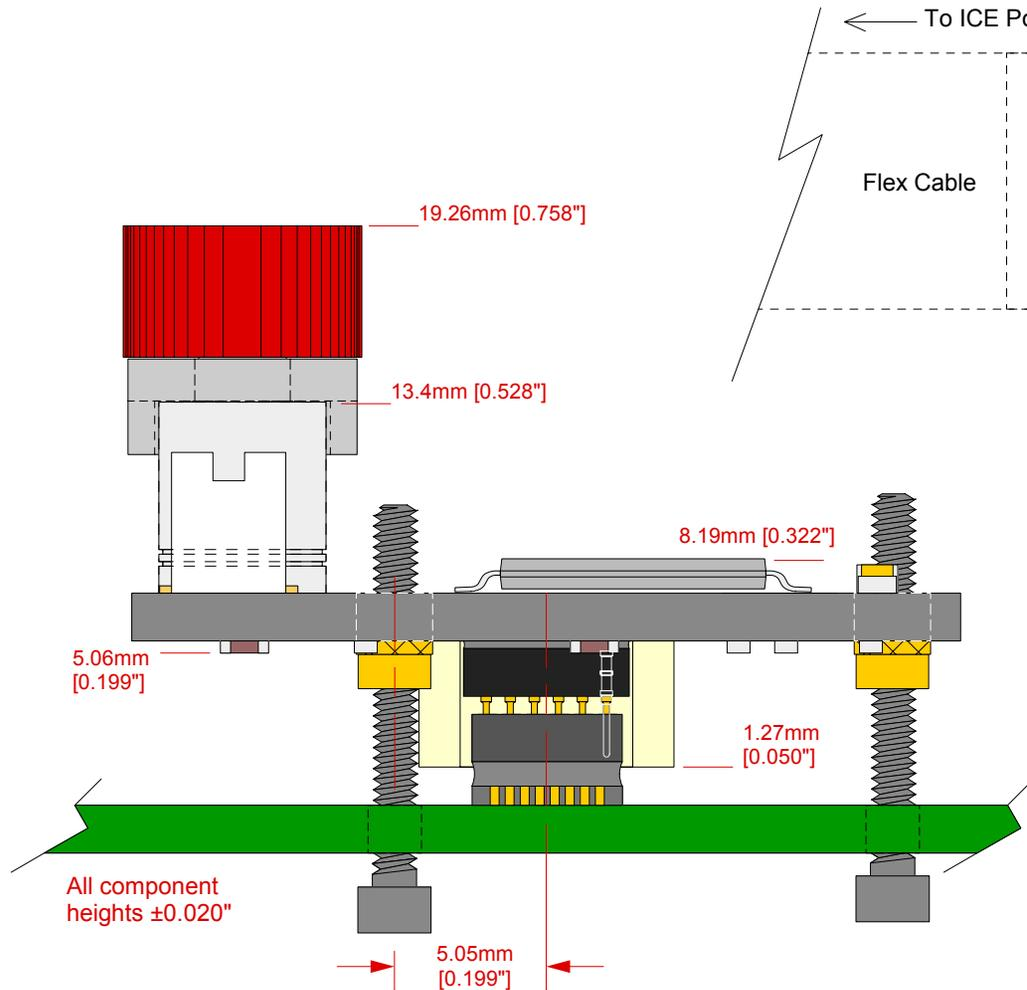
Side view: CY3250-21X34QFN Pod on QFN32 foot
