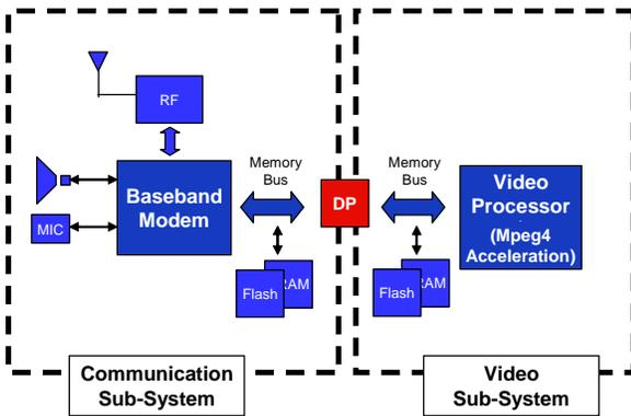
Figure 2. Example of a Handset Block Diagram, using a Dual-Port to Connect Two Subsystems
