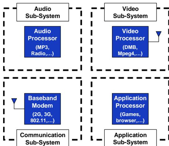
**Figure 1. Example of a Modular Architecture with 3 Subsystems**
