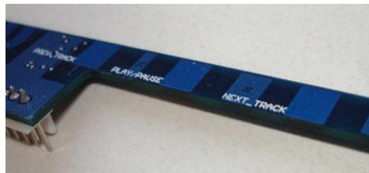
**Figure 2: Image of the top of the Multimedia board. Notice the gaps (Dark blue) between the ground fill and the sensors (lighter blue)**
