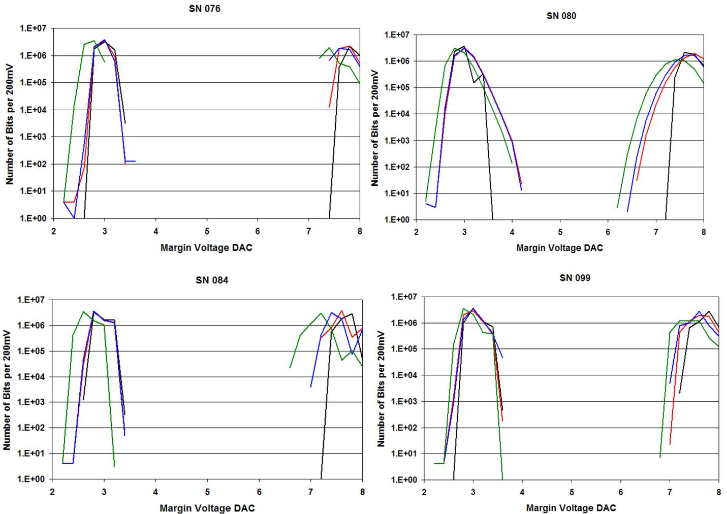
**Figure 14. Vt Distributions for Biased DUTs Irradiated to 10K, 20K and 30K rad(Si)**
