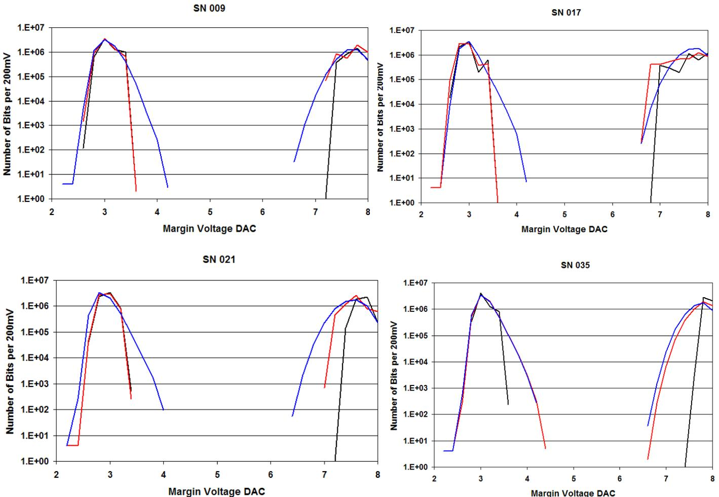
Figure 13. Vt Distributions for Biased DUTs Irradiated to 10K and 20K rad(Si)
