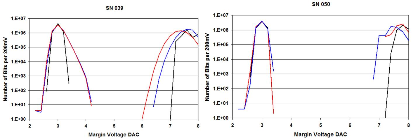
**Figure 15. Vt Distributions for UnBiased DUTs Irradiated to 20K and 50K rad(Si)**
