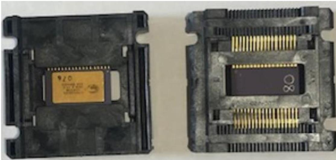
**Figure 2. 32 Pin Ceramic Flat-Packs in Plastic Carriers**
