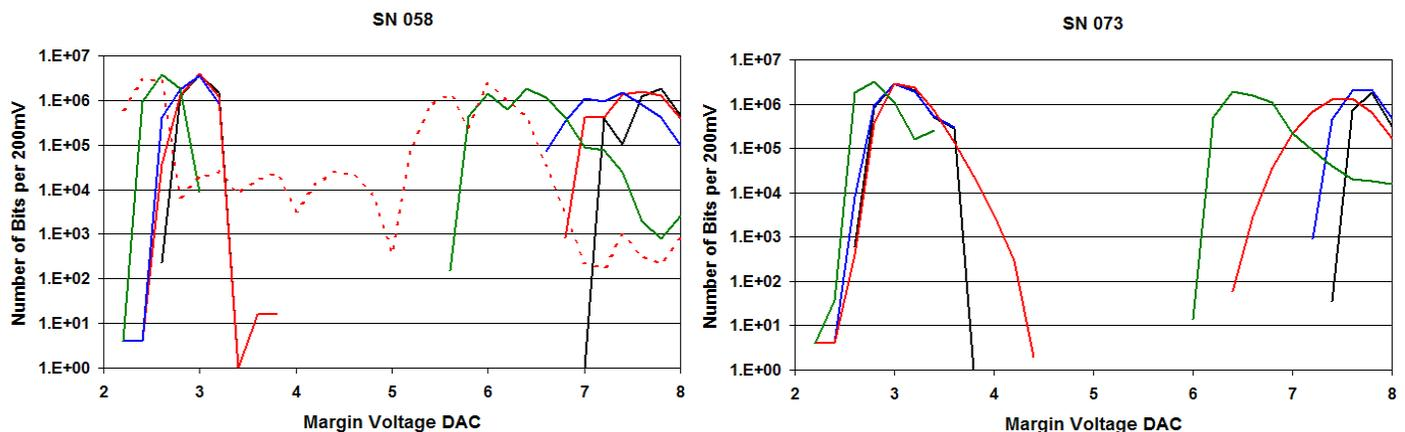
**Figure 16. Vt Distributions for UnBiased DUTs Irradiated to 20K and 50K rad(Si)**
