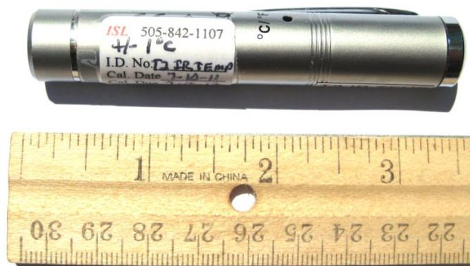
**Figure 3. I.R. Temperature Sensor**
