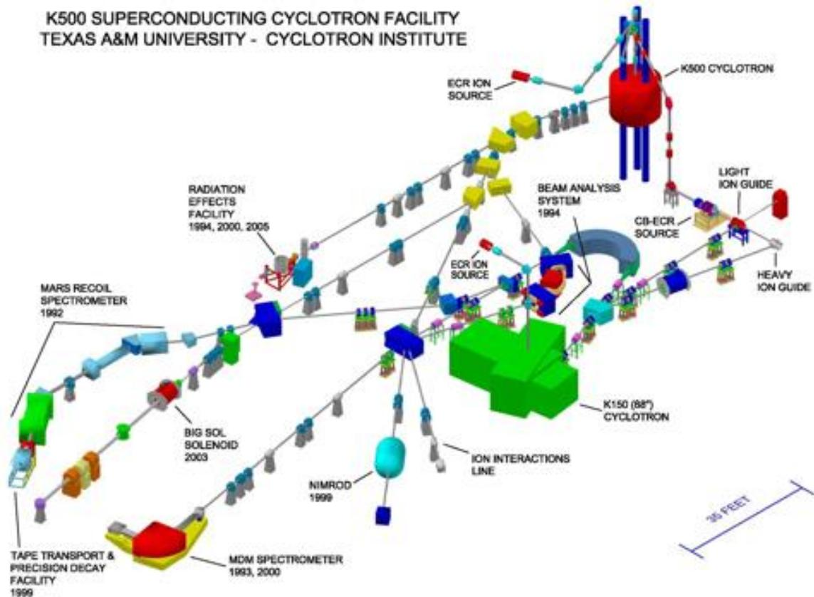
**Figure 4. Overview of Texas A&M Cyclotron Facility (TAMU)**
