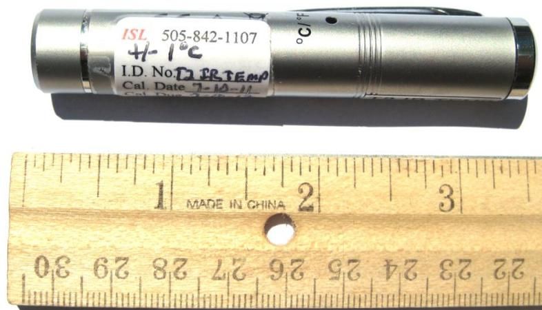
Figure 5. Infrared Thermometer
