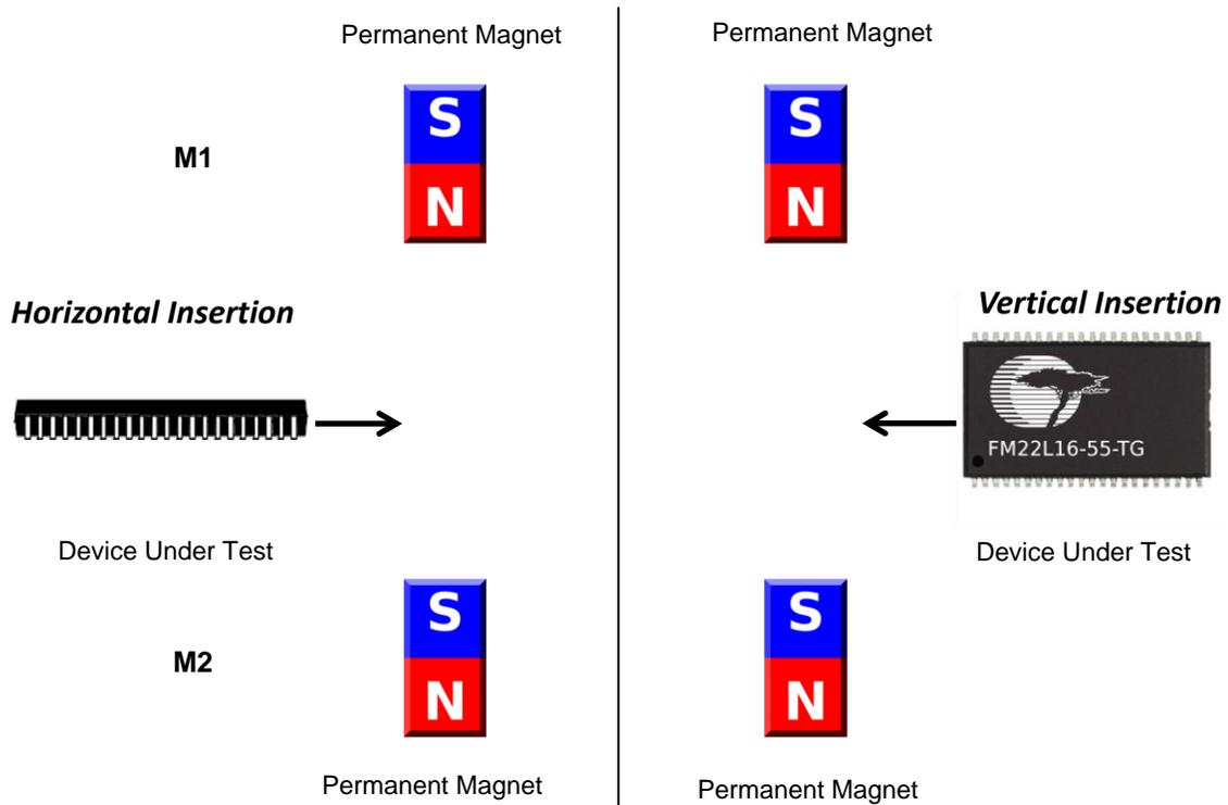
Figure 2. Magnetic Field Setup and Insertion Methods
