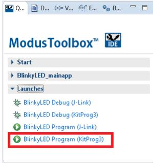
If needed, the IDE builds the application and messages display in the Console. If the build is successful, device programming starts immediately. If there are build errors, then error messages will indicate as such. When complete, the LED will start blinking.
