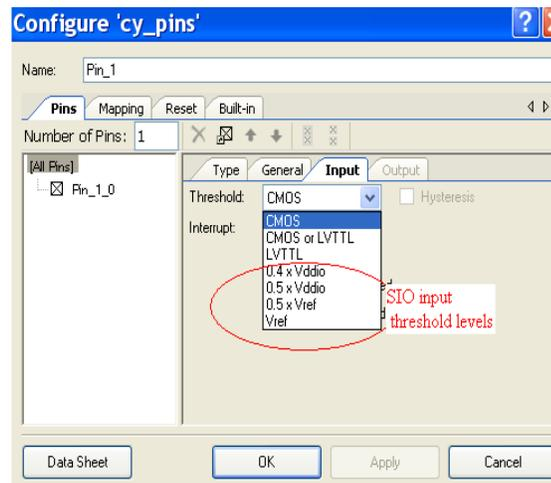
Selecting  $0.5 \times V_{REF}$  and  $V_{REF}$  threshold options add Reference Terminal to the Digital Input Pin component. This allows to route external reference from other components such as DAC or Pin.
