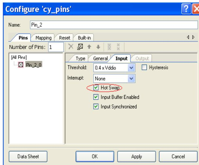
Use the hot swap capability to interface to peripherals that operate at different voltage levels. The following example shows how to interface to peripheral operating at 5 V while the PSoC 3 or PSoC 5LP device runs at 3.3 V. The SIO pin Drive Mode is configured to Open Drain, Drive Low mode.
