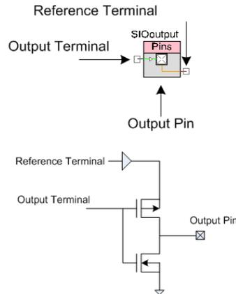
GPIO pins can source 4 mA and sink 8 mA; SIO pins can source 4 mA and sink 25 mA.
