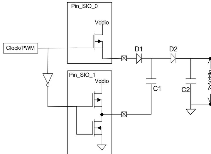
When the clock or PWM goes high, the Pin\_SIO\_0 charges the capacitor C1 to  $V_{DDIO}$  referenced against GND on the Pin\_SIO\_1. When the clock is low the Pin\_SIO\_0 is floating because of the open drain connection. But the low side of C1 is now  $V_{DDIO}$ ; this makes C1 to have a  $2 \times V_{DDIO}$  voltage developed at its high side. This makes the diode to conduct and thus charges the capacitor C2 to  $2 \times V_{DDIO}$ .
