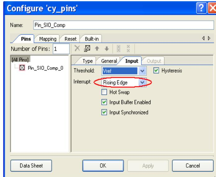
In the background loop, the device is put to sleep using `CyPmSleep()` API. When the SIO voltage crosses the reference, it generates rising edge at comparator output and wakes up the device from sleep. After wakeup, the device enters the ISR routine inside ISR and the interrupt flag is cleared. In the background loop, it toggles the pin `Pin_LED` before going to sleep again. The same code can be written for the hibernate mode too using `CyHibernate()`.
