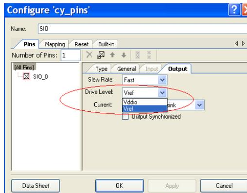
Select  $V_{REF}$  Drive Level option to configure the pin as SIO in regulated output mode. It adds reference terminal to the Digital Output Pin component. This allows to route external reference from other components such as DAC or Pin.
