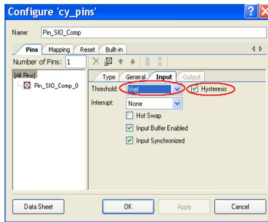
In the input tab, the threshold is set to  $V_{REF}$  and hysteresis is enabled. Hysteresis of  $\pm 50$  mV is provided on the SIO input buffer to remove the noise effects. The SIO\_HYST\_EN register enables the hysteresis individually for each SIO pin. See the TRM for more details.
