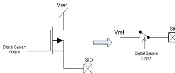
**Single Pole Double Throw (SPDT):** SIO pin drive mode is configured as Strong Drive. The digital output to the SIO connects or disconnects the SIO pin between  $V_{REF}$  and Gnd.
