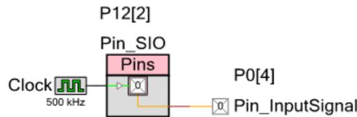
**Single Pole Single Throw switch (SPST):** SIO pin drive mode is configured as Open Drain, Drives High. The digital output to the SIO connects/disconnects the  $V_{REF}$  and SIO pin.
