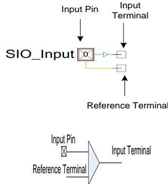
This component uses SIO pin if Hot Swap is enabled and threshold is set to anything other than LVTTTL or CMOS. **Note** The outline in pink indicates that the Digital Input Pin component uses SIO pin.
