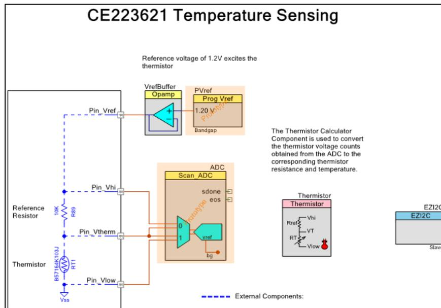
A 10-kΩ reference resistor is connected in series with the thermistor (B57164K103J).
