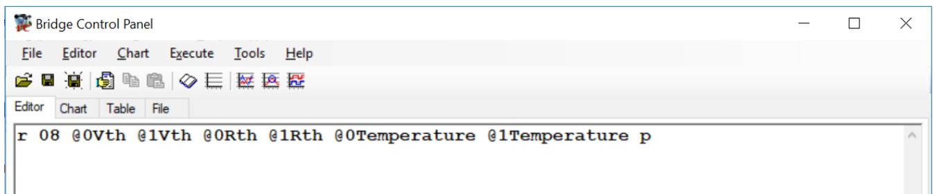
7. Click the read command on the **Editor** tab. Then click the **Repeat** button to read the sensor data continuously.
