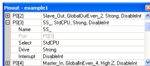
Figure 9. Example SS_ GPIO Configuration
