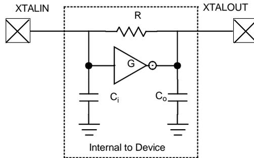
**Figure 3. Equivalent Circuit of a Quartz Crystal**
