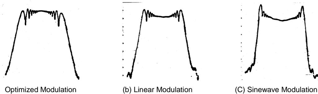
Why is a flat spectral profile optimal? The band of frequencies over which the EMI energy is spread is fixed by the modulation width used, it does not vary with the modulation profile. Because EMI testing is concerned with peaks, you have to spread that energy evenly over this frequency band. A flat spectral profile with minimal peaking shows that the energy is evenly spread across the frequency band.
