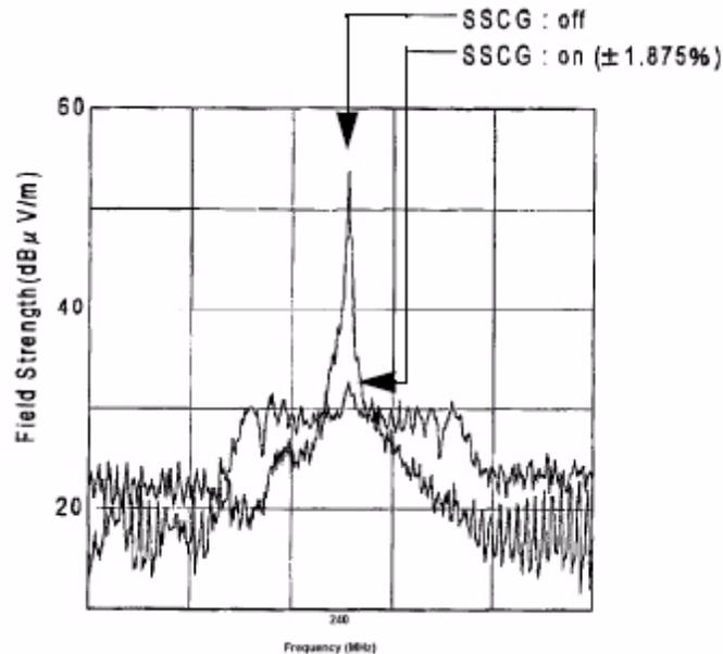
The SST technology was developed solely for the purpose of reducing peak EMI. It eases passage of regulatory testing, and reduces total manufacturing costs. Historically, EMI problems arise after a board is designed and its functionality is proven. If prototype boards failed EMI tests, EMC engineers would step in and adjust with component values, add some combination of chokes, more shielding or better gaskets to address specific frequencies at which the board failed.
