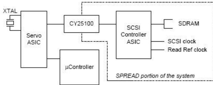
By implementing SST in the SCSI/SDRAM portion of the design, this customer achieved a significant (>10 dB for many harmonics) amount of reduction in the measured speak EMI of the system. Because the microcontroller is used in part for drive control timing circuitry, it does not work well with a SST signal, but if that function is migrated to the Servo ASIC, additional reduction can be achieved by using the spread spectrum to drive the  $\mu$ C as well.
