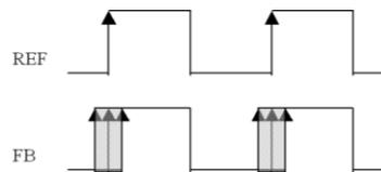
Figure 7 (a) and (b) show a comparison of an ideal and realistic downstream PLL performance when tracking an SST reference signal. In Figure 7 (a) the reference (REF) and feedback (FB) inputs to the phase detector are perfectly aligned and as the reference frequency changes the PLL loop responds instantly and the feedback signal perfectly ‘tracks’ the reference in phase and frequency.
