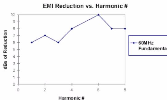
The same total amount of energy is still present; however, the peak value is reduced. In theory it would be possible to spread the signal so far that the energy density can be reduced all the way to thermal noise floor, in which case there would be no harmful emissions in the environment at all. Minimum signal to noise ratio requirements will of course dictate a higher level be used in practice.
