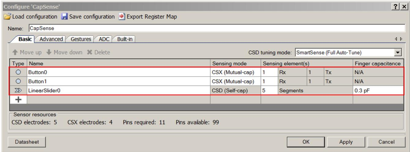
Figure 11. CapSense Configuration Window – Advanced / General
