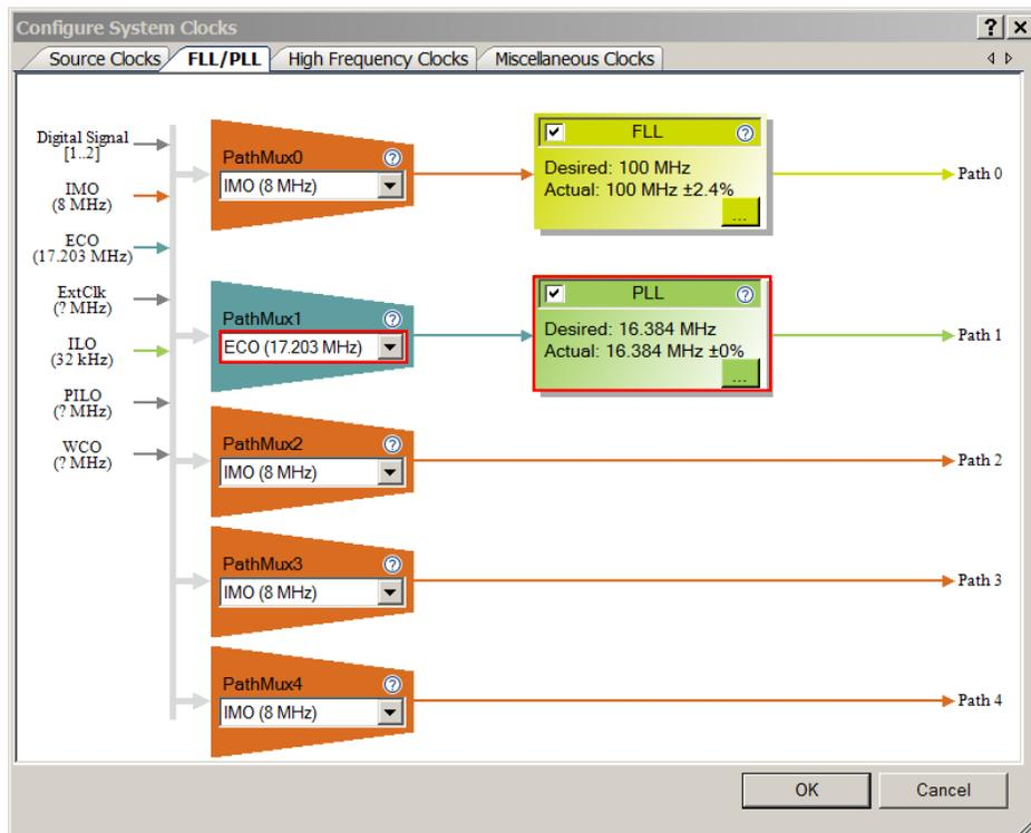
Figure 16. High Frequency Clocks Configuration
