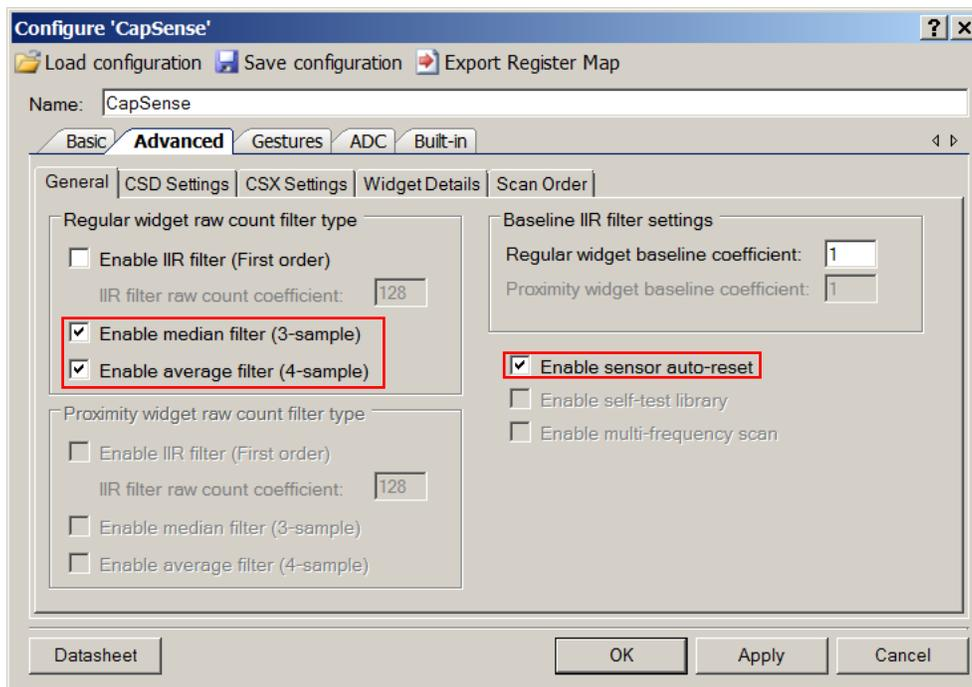
Figure 12. CapSense Configuration Windows - Advanced / CSD and CSX Settings
