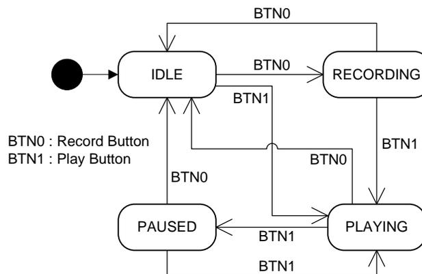
Each state is linked to a different icon displayed in the LCD. The Operation section shows the screenshots of each state. The screen also shows the current volume in percent, and the time duration of the record/play. The GraphLCDIntf Component drives the LCD. It is configured to have an 8-bit wide bus. The example uses an open-source graphics library for embedded system called [µGUI](#). The firmware uses this library to draw text and figures on the LCD display.
