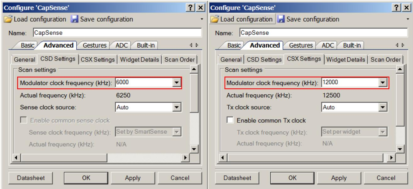
Figure 13. CapSense Configuration Window – Advanced / Widget details / Buttons
