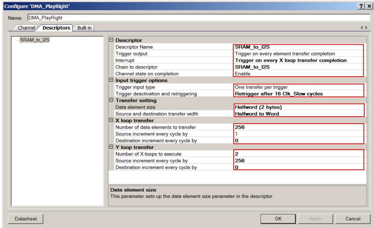
Figure 9. I2S Configuration Window
