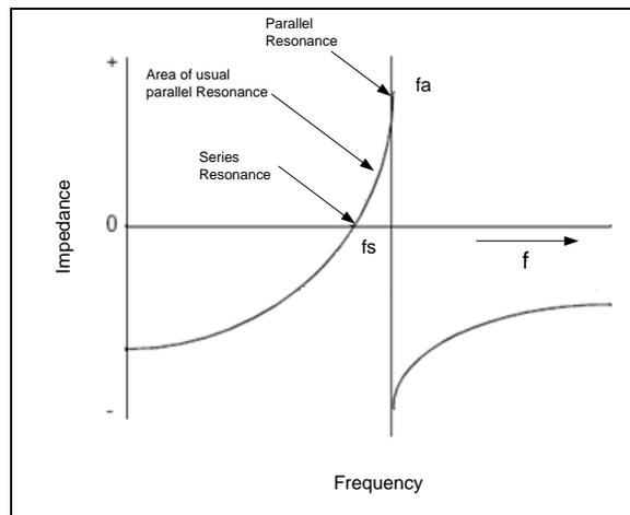
When a crystal is operating at series resonance, it looks purely resistive, and the inductive reactance of  $L_1$  equals the capacitive reactance of  $C_1$ . Since these impedances are  $180^\circ$  out of phase, they cancel out each other, leaving  $R_1$  as the impedance between the crystal terminals.
