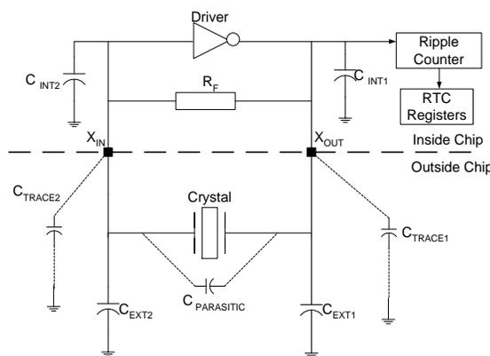
An equivalent load capacitance C<sub>EQ2</sub> on X<sub>IN</sub> pin can be defined as shown in Equation 6.
