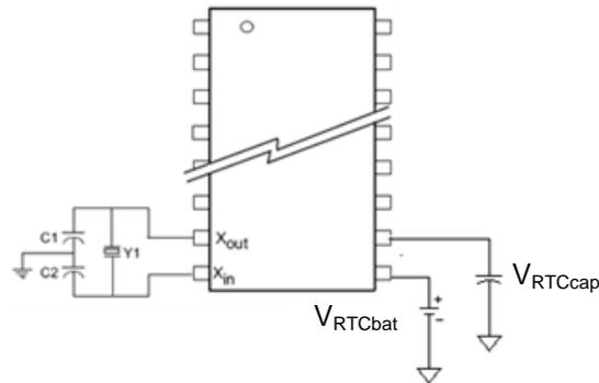
The load capacitances C1 and C2 are inclusive of the PCB parasitic components, including the capacitance due to the land pattern of crystal pads/pins, X<sub>IN</sub>/X<sub>OUT</sub> pads, and copper traces connecting crystal and device pins. Equation 9
