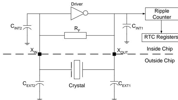
The Pierce-type oscillator uses a crystal that operates in parallel mode. The nominal frequency of oscillation for the crystal is defined under the specific load condition. To oscillate the crystal at its specified frequency, you should design the application board in such a way that the load capacitance across the crystal pads (X<sub>IN</sub> and X<sub>OUT</sub>) on the PCB is equal to the specified load for the crystal.
