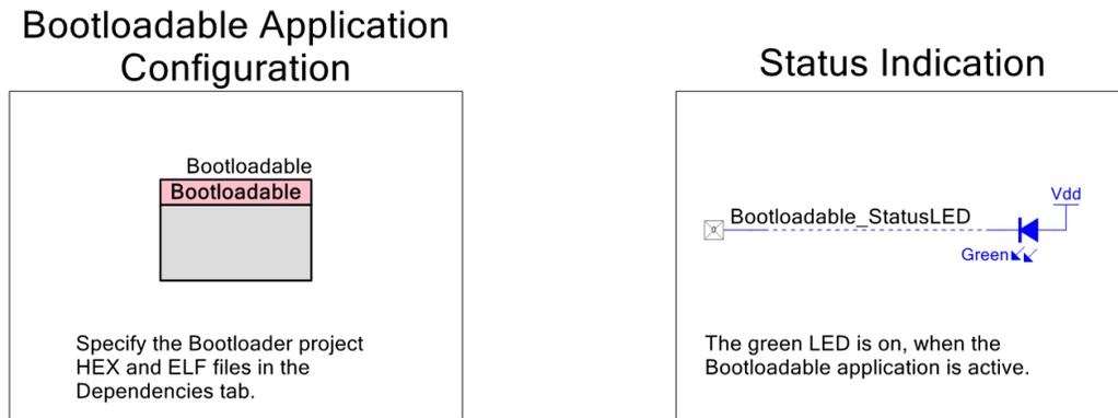
The Bootloadable project is an example of an application that can be downloaded and installed using the Bootloader. The Bootloadable Component defines and configures the Bootloadable project. You must specify the Bootloader project HEX and ELF files in the **Dependencies** tab of the Bootloadable Component to get information about the Bootloader project. This application enables the status LED, waits for a few seconds, and then returns to the Bootloader.
