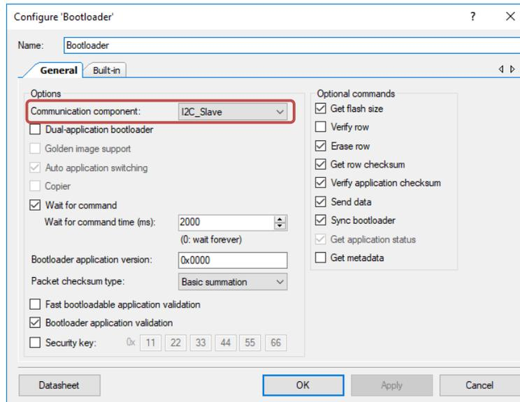
For the correct Bootloadable Component operation, associate your Bootloadable project with the HEX file of the Bootloader project. This way, the Bootloadable project gets the information about the Bootloader project (for example, properly calculates where it belongs in memory).
