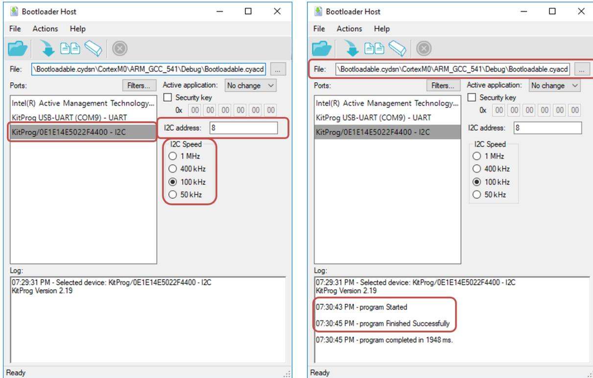
**Note:** To perform successful bootloading operation, the Bootloader on the target device must be active. Check the kit's blue LED's state and Press the kit's **Reset** button if the Bootloader is not active.
