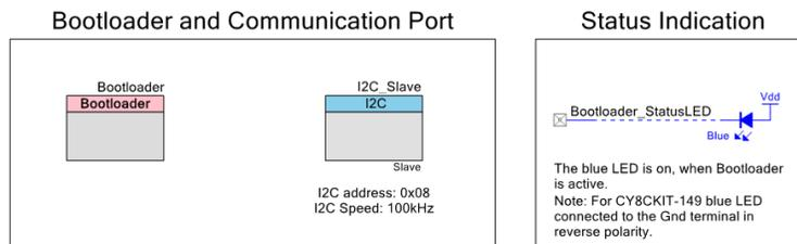
The Bootloader Component uses the I<sup>2</sup>C (SCB mode) Component configured in the Slave mode to communicate with the host. The Bootloader receives and executes commands from the host, then passes the responses to these commands back to the host; via the I<sup>2</sup>C interface. The Bootloader collects and arranges the received data and manages the actual writing of flash through a simple command/status register interface.
