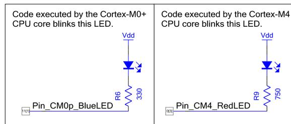
[Figure 2](#) shows the firmware design. Note that after PSoC 6 device reset, CM0 always executes first while CM4 is held in a reset state. PSoC Creator automatically generates code in `main()` for CM0 (file `main_cm0p.c`) to enable CM4.
