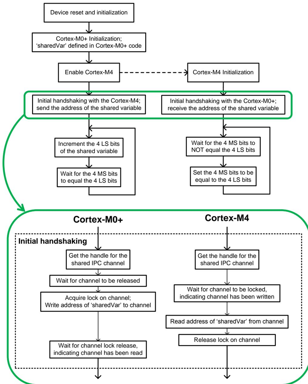
In the main() functions for both CPUs, the shared variable is never accessed directly. Instead, utility functions provide mutex lock and release access for reading and writing the variable. These utility functions in turn call PDL IPC driver functions that provide an atomic IPC channel lock and release capability. This ensures that only one CPU at a time accesses the shared variable.
