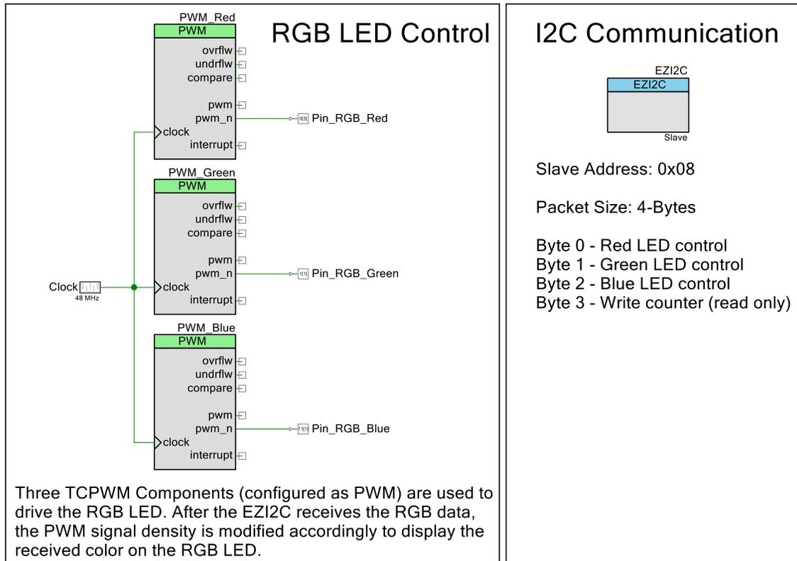
In this example, the EZI2C is configured with a 4-bytes buffer (memory), which can be accessed by the I<sup>2</sup>C master. The first three bytes are writable and hold the red, green, and blue LED intensity and the fourth byte, which is read-only, holds the number of Write operations performed after the device reset.
