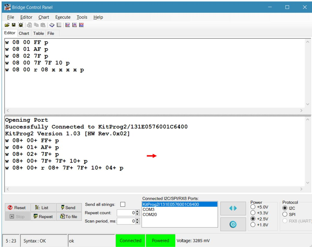
3. Select **Tools > Protocol Configuration**, navigate to the **I2C** tab, and set the **I2C speed** to '100 kHz'. Click **OK**. BCP is now ready for reading and displaying the sensor data. For the testing procedure, see [Operation](#).
