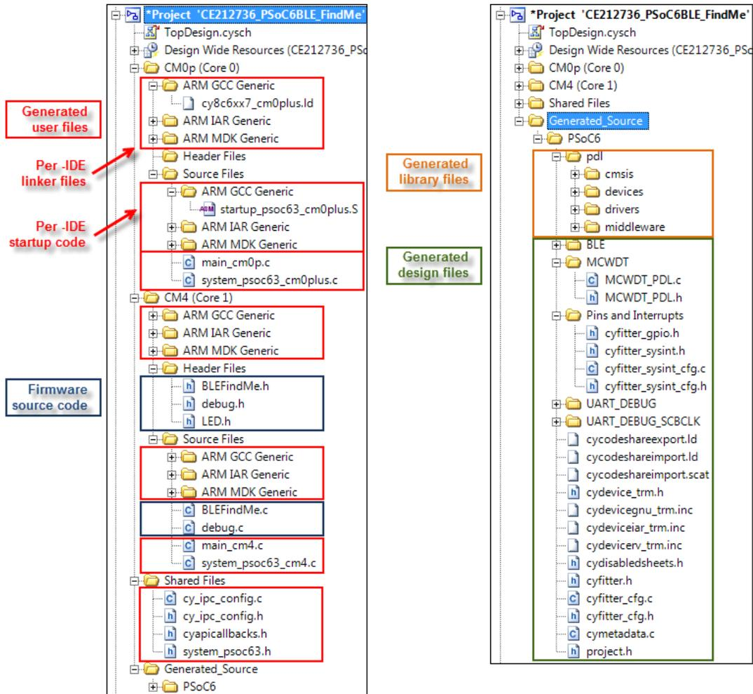
The *Generated\_Source* item in the Workspace Explorer pane contains all the files that are in the project's *cydsn/Generated\_Source* folder. This design uses a BLE Component, a multi-counter watchdog timer (MCWDT), and a UART to print debug messages to a terminal window. It also has pins to control LEDs, and sets up system interrupts.
