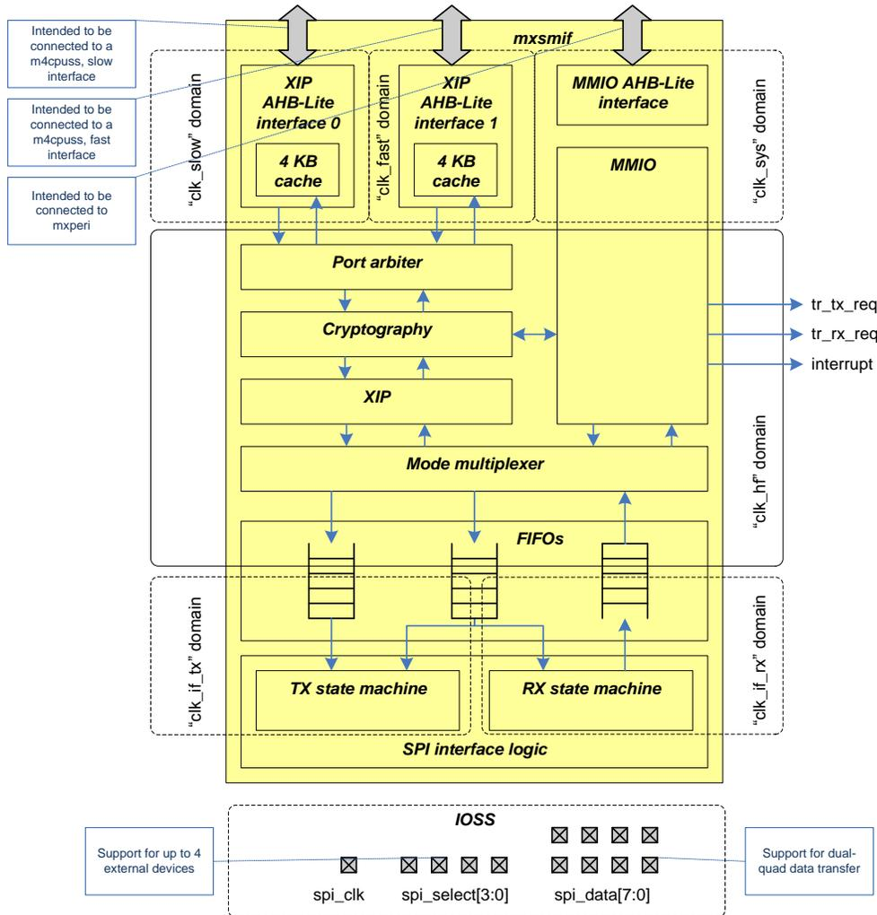
See the Serial Memory Interface (SMIF) section in the device *Technical Reference Manual (TRM)* for more information about the hardware block description and configuration values.
