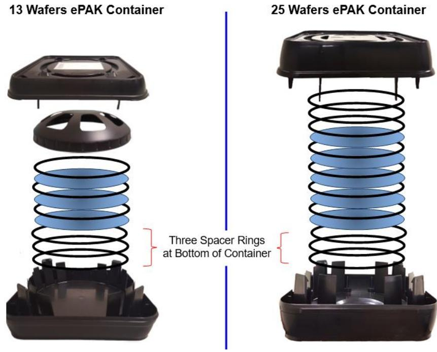
4. For packing 300-mm-diameter F-RAM wafers, use one compliance ring and one spacer ring at the bottom of the container to prevent the bottom wafer from contacting the bottom wall of the container.
