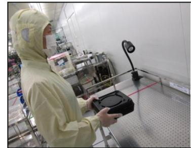
4. Open the F-RAM wafer container in a clean room area on a well-lighted work table. The area should have an ionizer running, and the operator must have a vacuum wand and ESD grounding.
