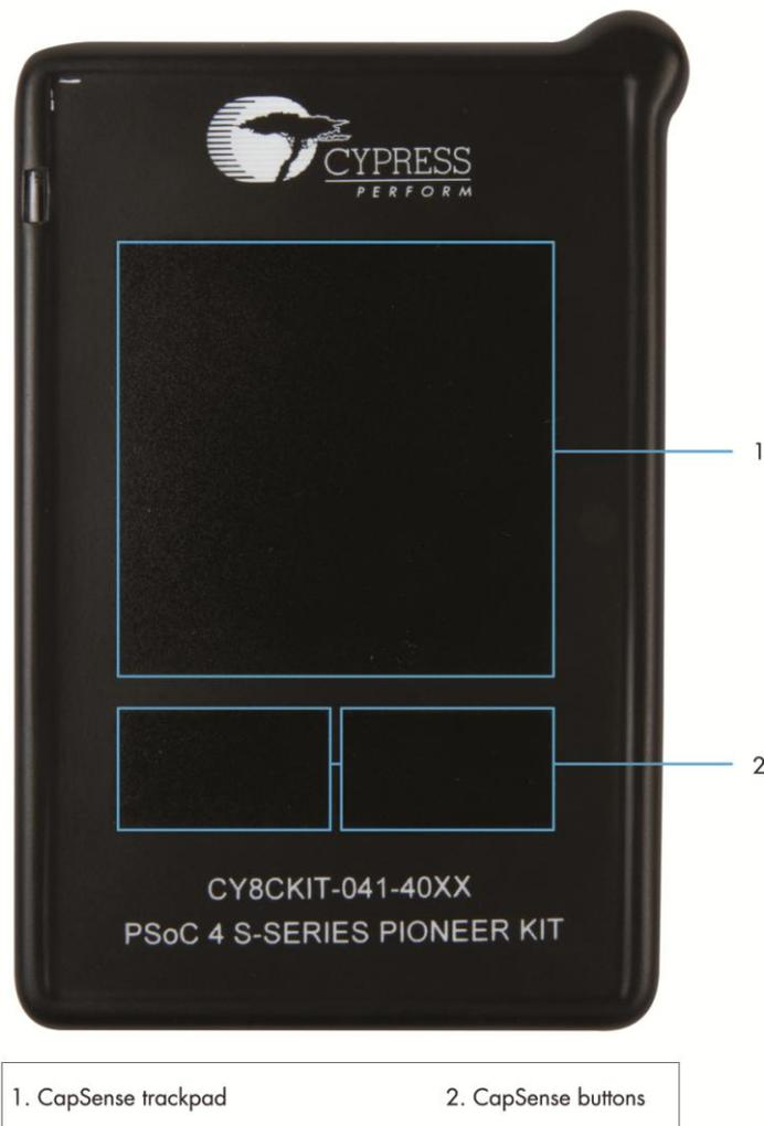
Note: The above figure shows the kit without the Overlay
