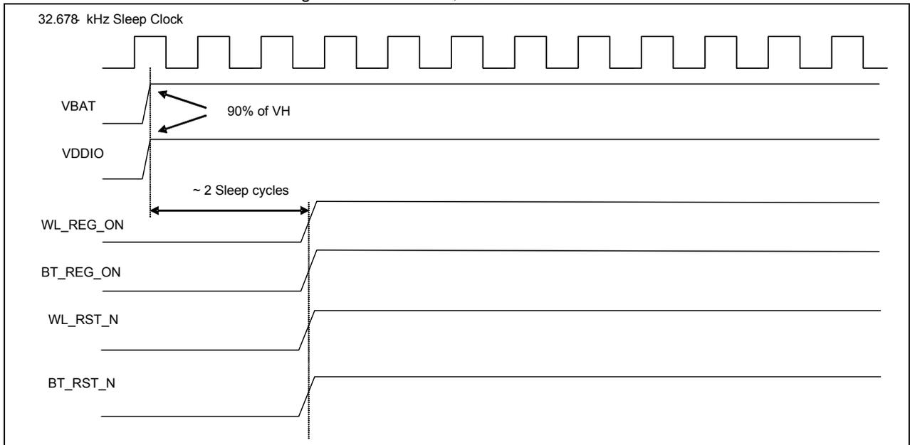
Figure 7. WLAN = OFF, Bluetooth = OFF
