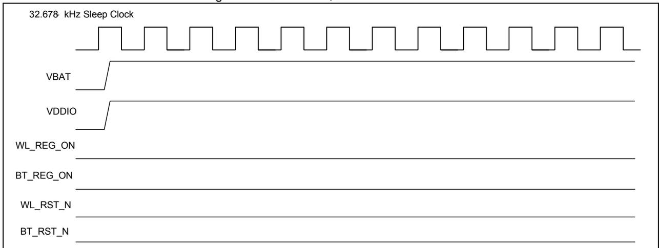
Figure 8. WLAN = ON, Bluetooth = OFF
