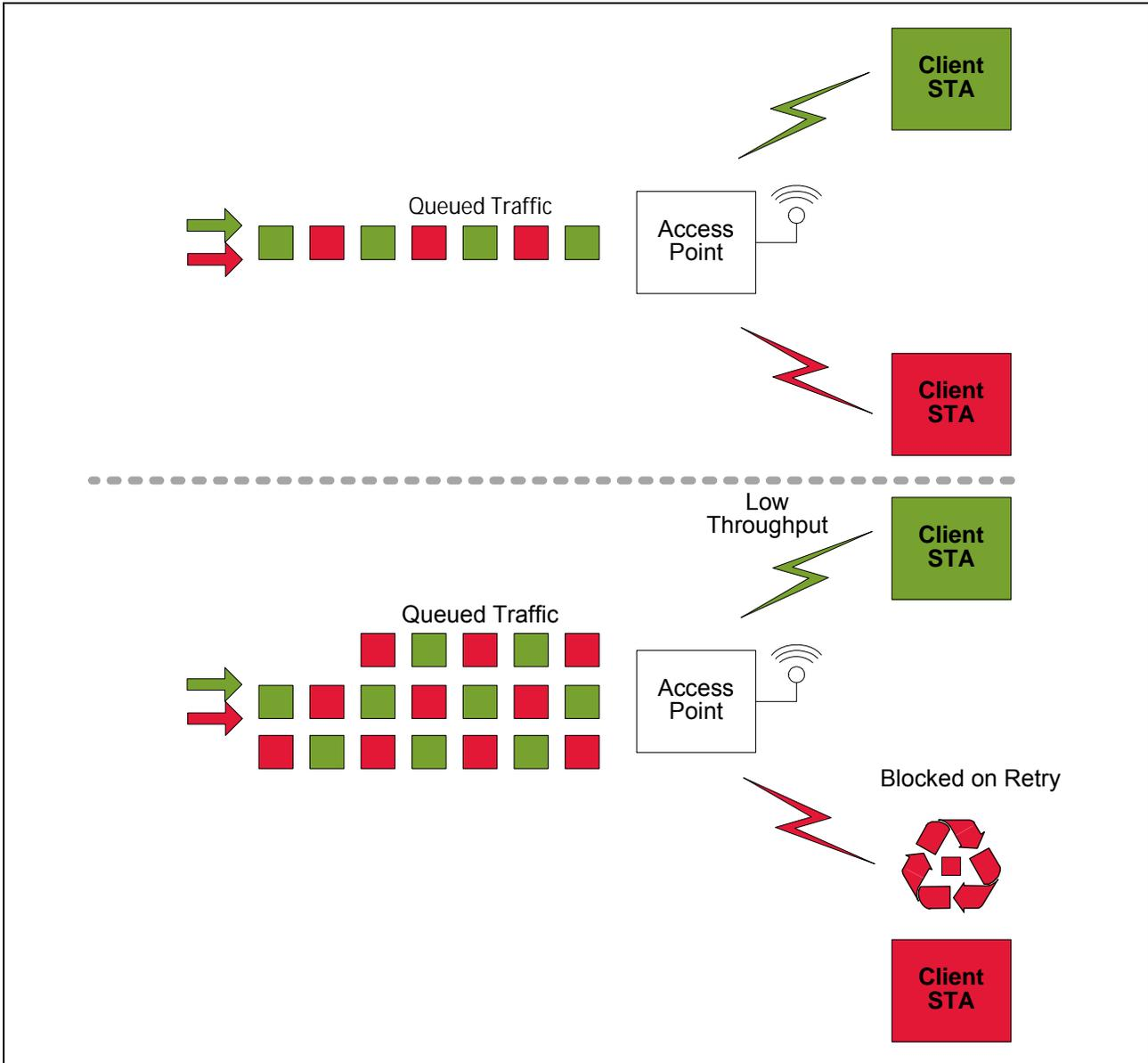
Using Pspretend suspends the bad link: no further data is transmitted to it—instead, the data is queued for later transmission and the existing good link continues to work normally, unaware of the problem (Figure 3 on page 10).
