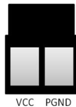
**Figure 3: Power connector X6**
