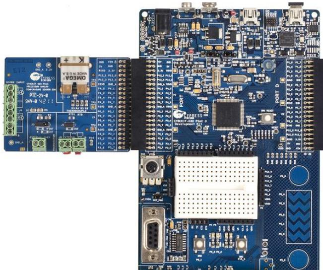
2. On KIT-025, ensure that there are wires shorting the terminals of J8 and J9, as [Figure 3](#) shows.
