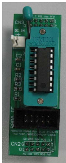
Figure 3-5: Place MCU on Adaptor Board
