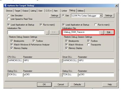
A typical debug initialization script may look like the following code. The necessary trace ports and pins enable is highlighted in dark red bold characters. These lines enable the port pins for trace. Note that at Port 0 also the JTAG pins have to be kept (write  $0 \times 0.0003$  FF).
