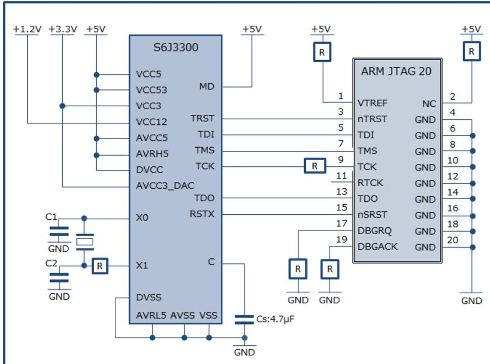
These devices have user mode and serial write modes. Figure 1 shows the user-mode connection. Serial write modes use P1\_05 and P1\_03 with the MD port. Table 3 lists the operation modes. This shows operation mode combination with MD port, P1\_05, port and P1\_03 port.
