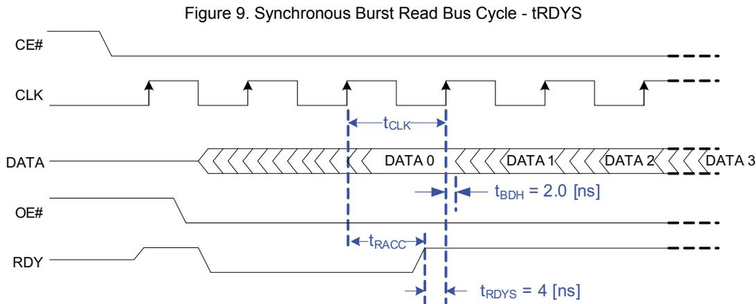
This minimum time for  $t_{RDYS}$  is defined by taking the minimum allowed clock period,  $t_{CLK}$ , and subtracting the maximum data RDY assertion time,  $t_{RACC}$ .
