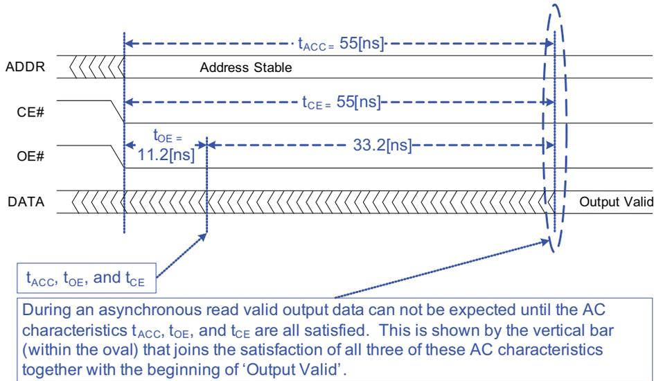
In Figure 4 valid read data can not be expected by 11.2 [ns] after OE# goes low. The output data will not be assured valid until 55 [ns] after CE# and OE# both go low. This is because  $t_{ACC}$  and  $t_{CE}$  must also be satisfied. The blue oval around the vertical bar emphasizes that all three AC characteristics must be satisfied before valid read data can be expected. Even if OE# went low as much as 43.8 [ns] after CE# went low it still would not make the read data become valid any earlier.
