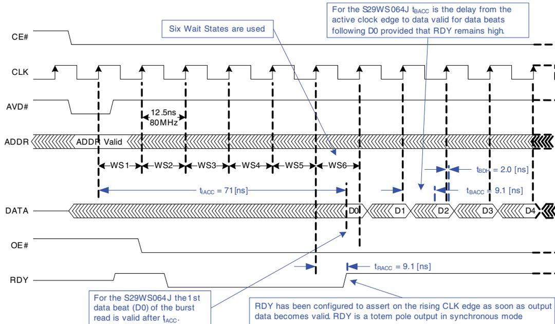
Burst Read performance is increased by minimizing the number of wait states needed for the first read of data, D0. Every active clock edge from AVD# low until D0 is valid is another wait state. In Figure 8 the number of needed wait states is 6. D0 becomes valid during WS6.
