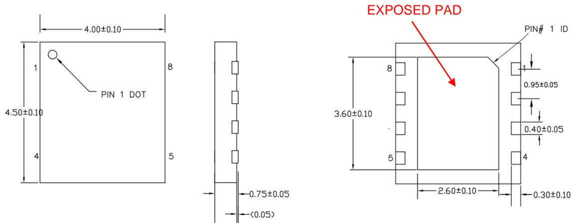
The I<sup>2</sup>C F-RAM EXPOSED PAD is not connected to the die and hence should be left floating. Ensure that the EXPOSED PAD of the I<sup>2</sup>C F-RAM DFN package is not soldered on the PCB when migrating to I<sup>2</sup>C F-RAM. Soldering it will cause the I<sup>2</sup>C F-RAM die to be exposed to excessive heat, which can result in bit failures and margin loss.
